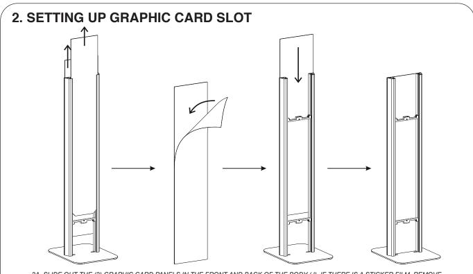
2A. SLIDE OUT THE (2) GRAPHIC CARD PANELS IN THE FRONT AND BACK OF THE BODY (J). IF THERE IS A STICKER FILM, REMOVE THAT FIRST. IF YOU HAVE PRINTED OUT A STICKER GRAPHIC, PLACE IT ONTO THE PANEL. IF YOU ARE USING A COMPLETE NEW PANEL, YOU CAN REPLACE THE INITIAL PANELS THAT CAME WITH THE FLOOR STAND. PLACE ONE PANEL BACK FIRST, THEN THE OTHER.
