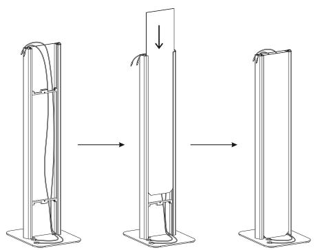
3A. WITH ONLY (1) PANEL BACK IN, SLIDE IN THE POWER CORDS AND ANY OTHER CORDS THAT WOULD NEED TO BE CONNECTED TO THE TABLET THROUGH THE BODY AS SHOWN. THERE WILL BE GAPS AT THE TOP AND BOTTOM FOR THEM TO ROUTE OUT TO THE POWER SOURCE AND TO THE DEVICE. SLIDE IN SECOND PANEL WHEN ROUTING IS FINISHED.
