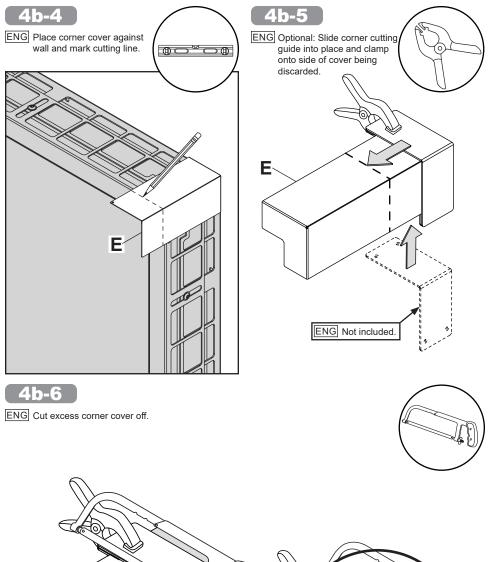
ENG Do not clamp fixture on wrong side of cutting line.
