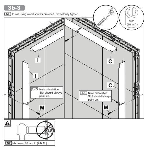
ENG Slide wall brackets in slot until they sit 1.25" from display guiding lines. Level and tighten wood screws. Repeat for left side.
