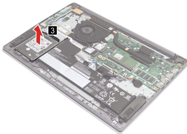
Figure 11. Disconnect the storage drive cable and remove the storage drive with bracket
