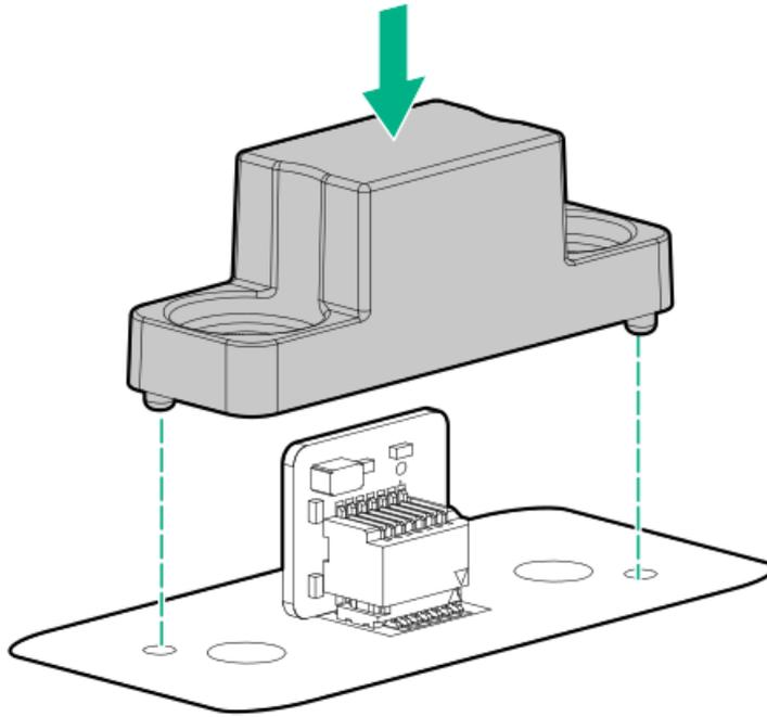
4. Secure the rivets into place by pushing them firmly through the holes in the TPM cover.
