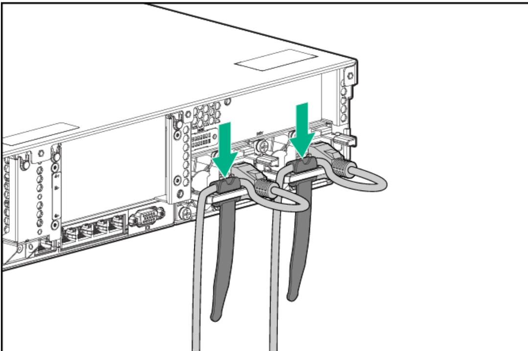
4. Secure the cables to the cable management arm.
