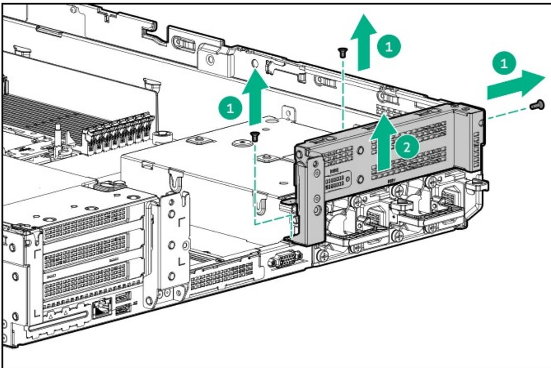
7. Install the drive cage compatible rear wall.
