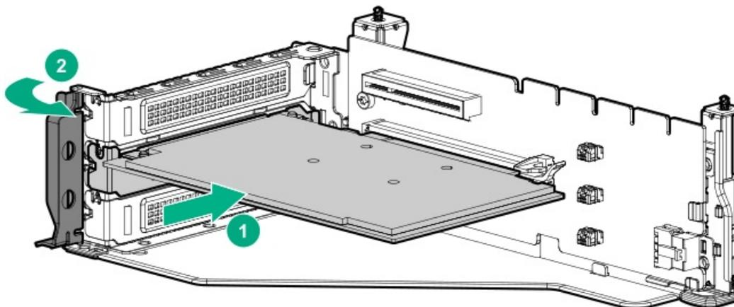
7. Install the PCIe riser cage into the server.
