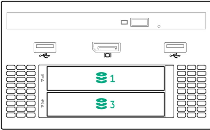
If a 2 SFF drive cage is connected to SAS expander port 3, then the drive numbers are 1 and 3.
