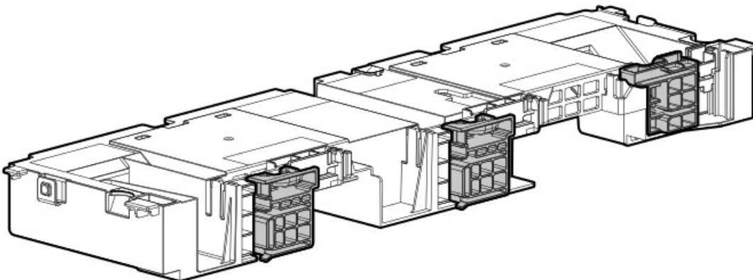
7. If the total maximum power requirement of all installed accelerators is higher than 25 W, install the high-performance fans and heatsinks to maintain proper system cooling:
