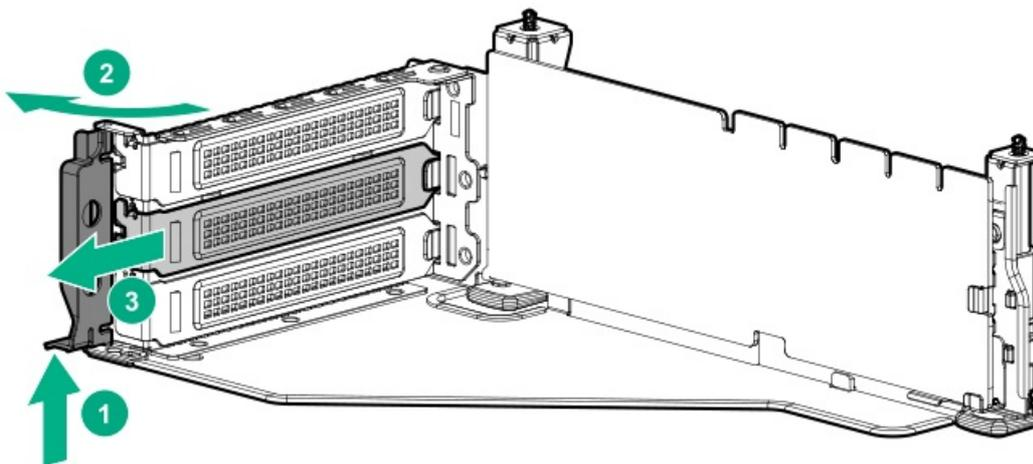
11. Install the accelerator into the secondary riser.
