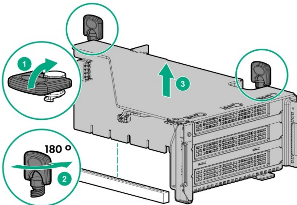
8. Locate slot 3, and then remove the expansion slot blank.
