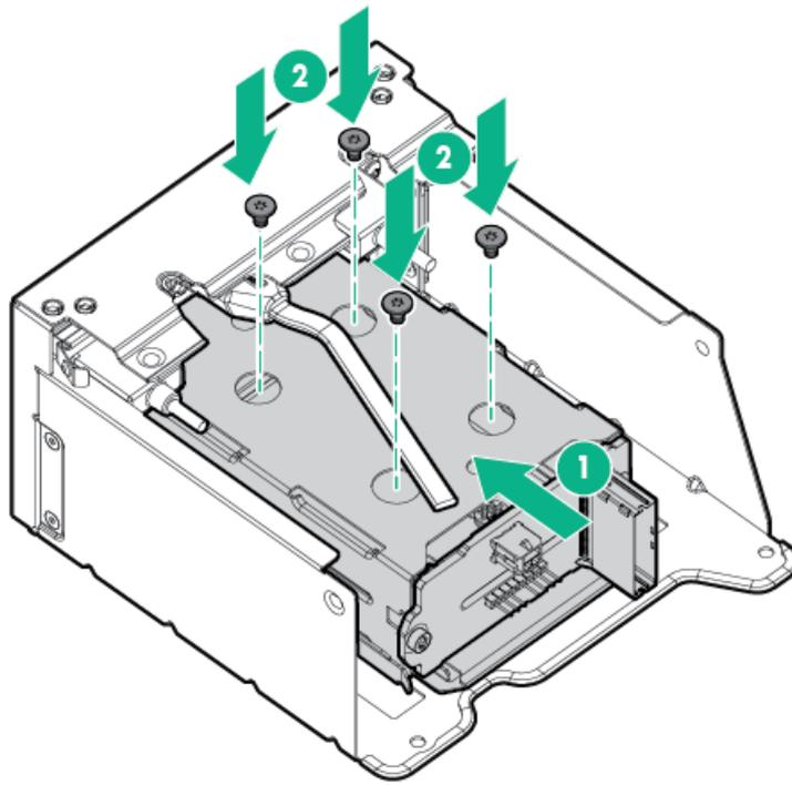
9. Install the optical disc drive tray.
