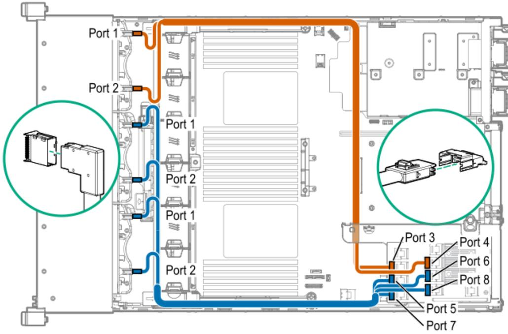
**Cable routing: 24 SFF drive options (box 1, box 2, and box 3 to SAS expander card and HPE Smart Array P816i-a SR Gen10 Controller, ports 1-2)**
