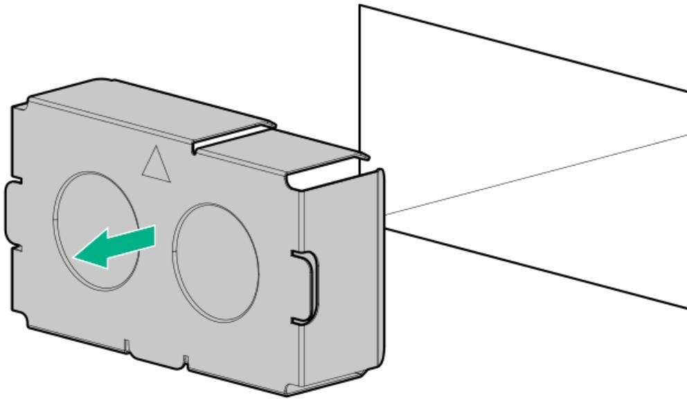
2. Remove the clear plastic cover on the side of the power supply.
