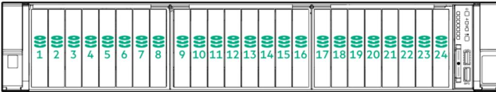
When any stacked 2 SFF drive cage is connected to the SAS expander, the drive numbering skips the second number. For example, when a rear 2 SFF drive cage is connected to SAS expander port 9, then the drive numbers are 25 and 27.
