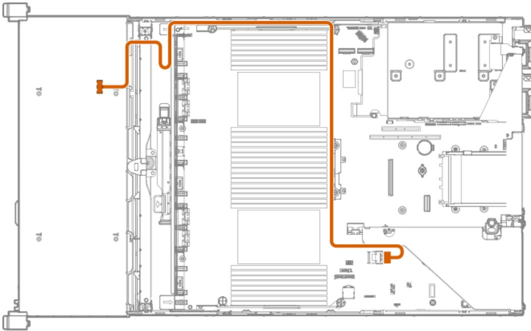
**Cable routing: Front 8 SFF drive options (box 1 to HPE Smart Array P816i-a SR Controller, ports 3-4)**
