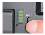
Power indicator button: Press this button to display the power, otherwise the power is not displayed. Electricity in more than 75% bright 4 lights, more than 50% light 3 lights, more than 25% bright 2 lights, more than 5% light 1 lights, if all the lights are not bright means the lack of electricity ,so you need to charge.
