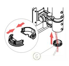
4B. Once all the wiring has been routed, use the end cap and canopy for a clean and organized seamless look. Click together the two pieces (G) and insert them in the bottom end as shown.
