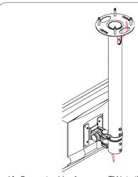
4A. Connect cables from your TV into the pole body as illustrated. Continue wiring through the body until the cable comes out from the hidden cutout in the ceiling into whatever connection is made (by others).
