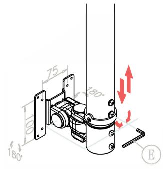
Turn screw with allen key (E) to loosen, then extend or retract pole to adjust to the desired height. Turn pole knob clockwise to tighten.
