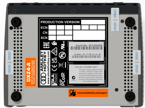
Figure 42: Location of the anti-tamper seals (not ZeroTop)
