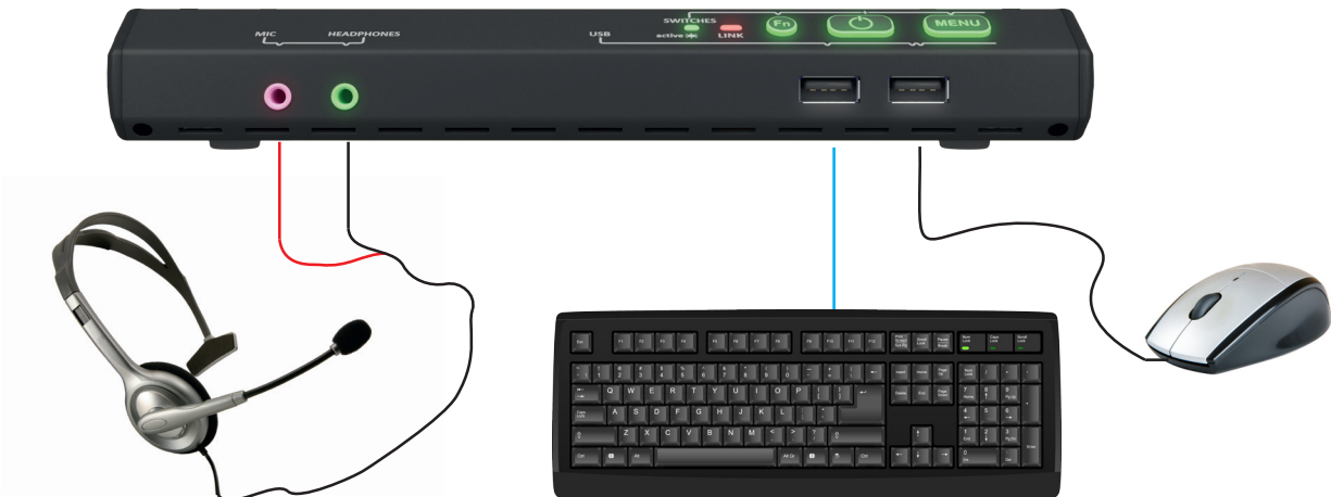
Figure 18: Front panel connections for the DXZ4 series
