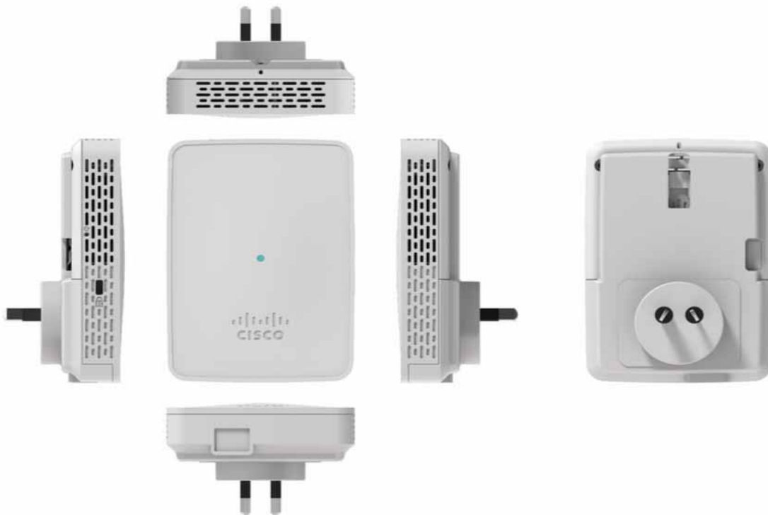
Figure 11 Sensor with AC Cradle for AU Region
