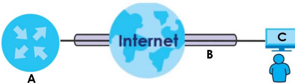
Figure 30 Example of NBG6818 Acting As VPN Server
