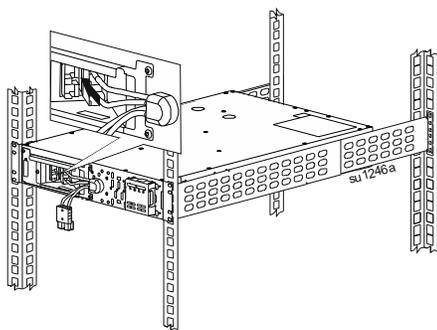
6 Connect the red color internal battery connector to the red color receptacle in the battery module. Be sure that the connection is secure.
