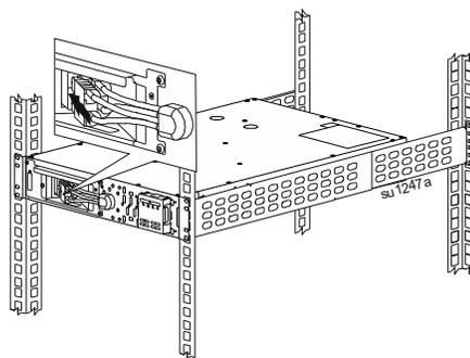
**NOTE:** Pull the strap provided on the connectors for disconnecting the battery. **Do not** pull the wires.
