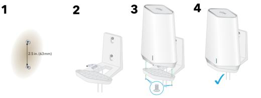
Note: When the screws are placed correctly, the holes at the back of the mounting bracket fit over the protruding screws, allowing you to slide the mounting bracket downward until the tops of the slots are resting on the screws.
