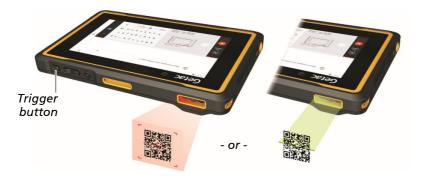
4. Upon a successful scan, the scan beam turns off and the decoded barcode data is entered in the Google Search bar.
