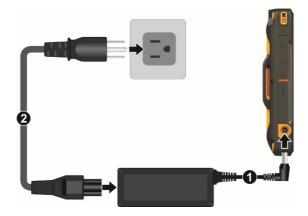
The charge indicator glows in amber when charging is in progress. Do not disconnect your device from AC power until the battery is fully charged, as indicated by the amber indicator turning into green. This will take a couple of hours.
