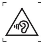
Figure 1 – Warning label (IEC 60417-6044)
