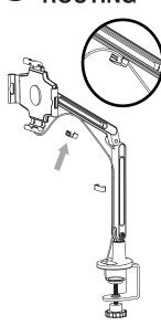
When routing cables for the from device to the power source, use provided clips as shown to keep the cables organized and tight to the arms to avoid any slack.
