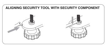
2B. Align the (2) dimples on the underneath of the security tool into the two holes on the security component on the clamp as shown above
