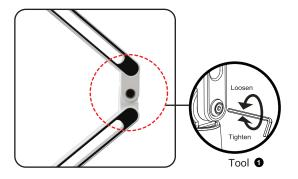
Each hinge of the product can be adjusted easily with the provided smaller allen key tool. Loosen to adjust and securely tighten after preferred position is set.
