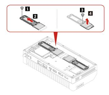
Note: After installing the new M.2 solid-state drive, ensure that you attach the new thermal pad to the new M.2 solid-state drive.
