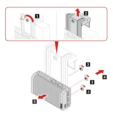
**Note:** When installing the Z hook kit, fasten the screws correctly to ensure that the computer is stable.
