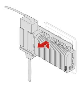
Remove the power cord from the power adapter. See "Power adapter and power cord" on page 38.
