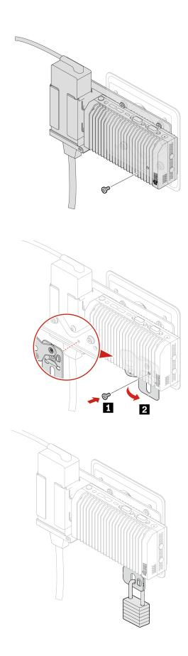
The replacement steps also apply to the computer with an IO expansion box installed. See "IO expansion box" on page 39.
