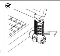
Adjust the locking tip according to the lock slot specification of your device.
