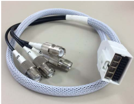
Figure 12 AIR-CAB002-DART-R= DART Connector
