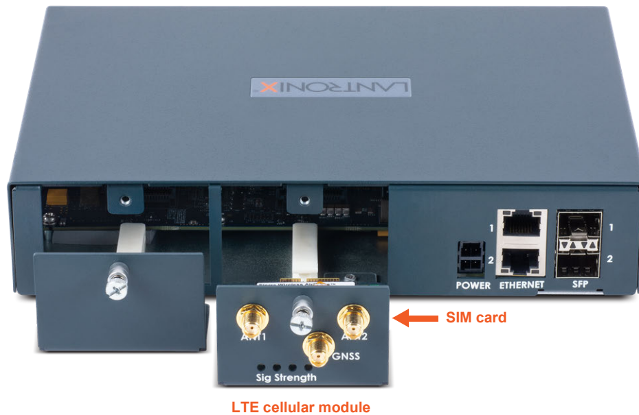
Figure 2-12 EMG 8500 LTE Cellular Modem Module
