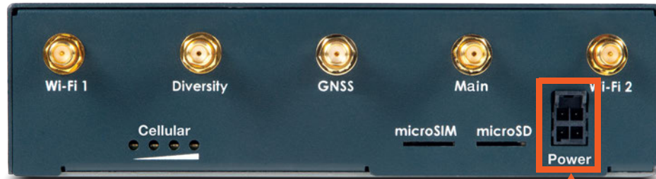
Figure 4-9 EMG 7500 Power Input
