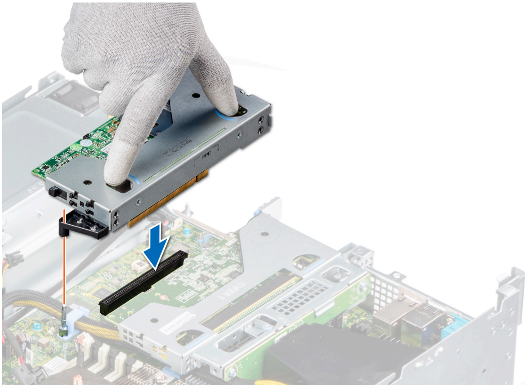
Figure 69. Installing the riser 2
