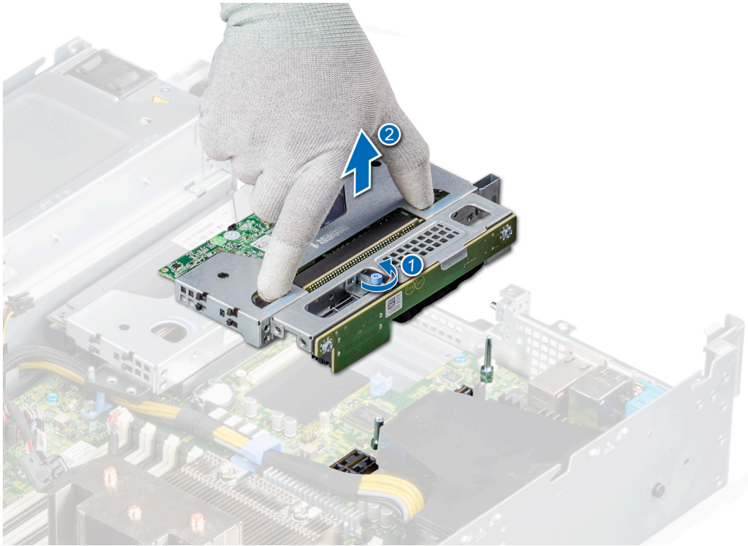
Figure 67. Removing the riser 1A
