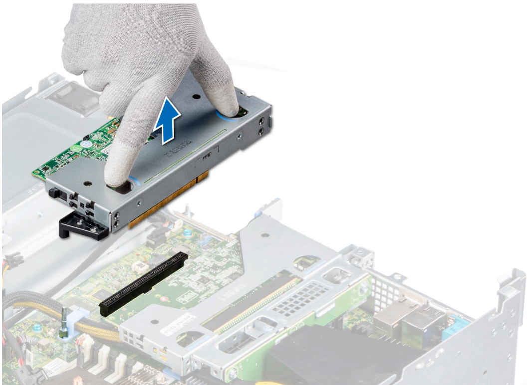
Figure 66. Removing the riser 2
