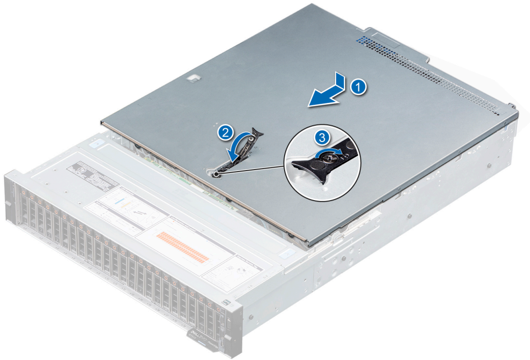
Figure 20. Installing the system cover
