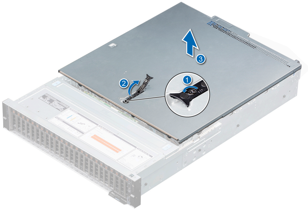
Figure 19. Removing the system cover
