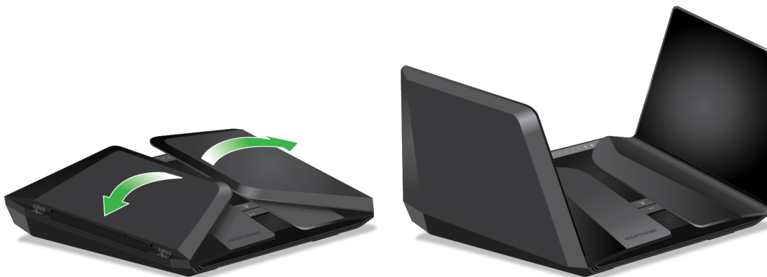
Figure 4. Position the antennas
