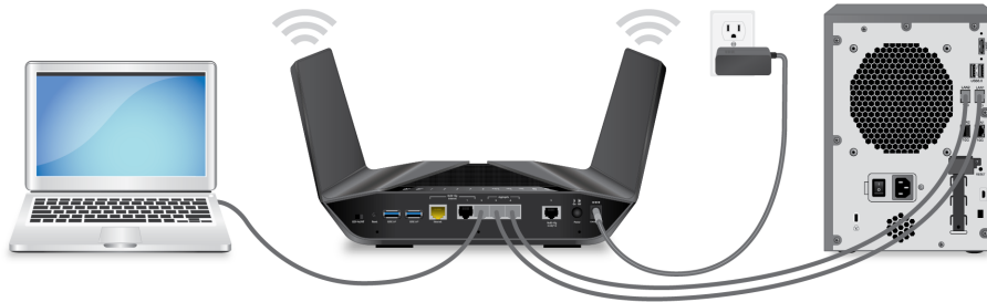
Figure 8. Ethernet port aggregation to a LAN device
