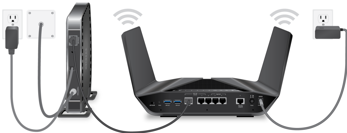
Figure 6. Router connected to a modem
