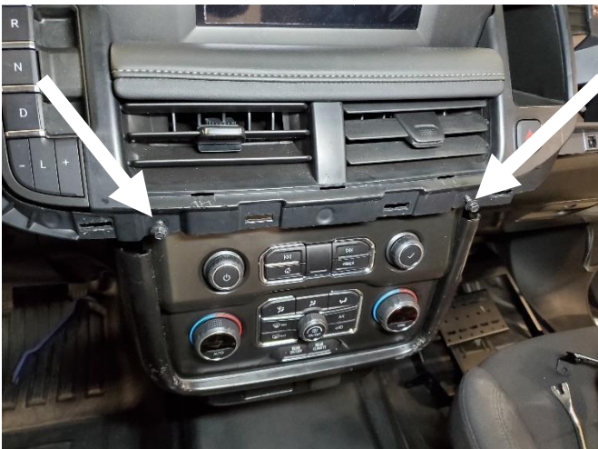
Remove 7mm head fastener found behind previously removed trim.
