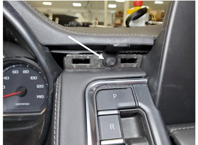
Attach upper dash mounting bracket as shown on driver side using previously removed fastener.
