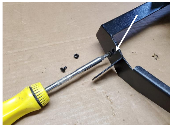
Attach the DMM frame to frame mounting brackets using 10-32 x 3/8" screws and keps nuts.
