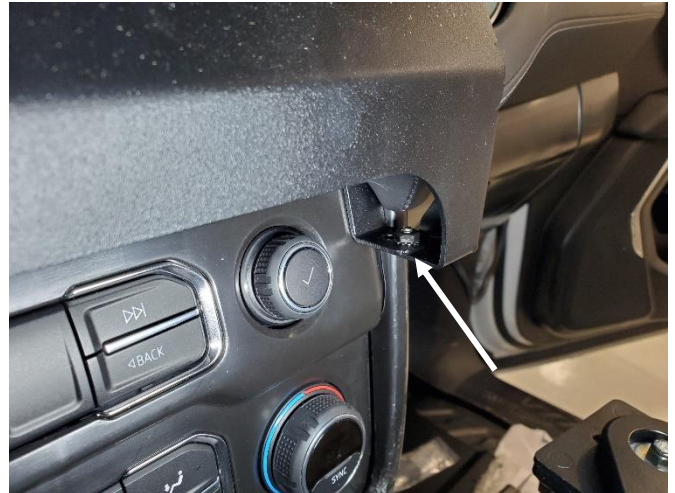
Attach to DMM frame to lower dash mounting brackets using 10-32 x 3/8" screws and keps nuts.
