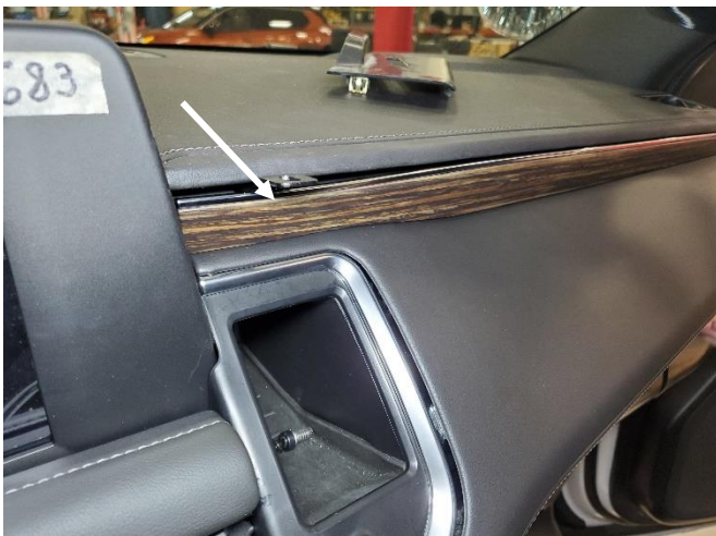
Snap upper passenger side dash trim back in allowing mounting bracket to stick out the top.
