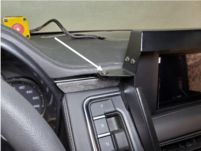
Place DMM frame on upper dash mounting brackets and attach using 10-32 x 3/8" screws and keps nuts.
