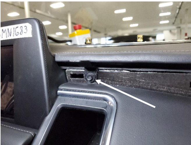
Attach upper dash mounting bracket as shown on passenger side using previously removed fastener.
