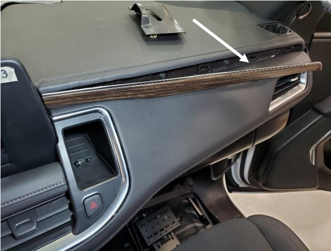
Remove upper dash trim on passenger side by gently prying with a panel removal tool.
