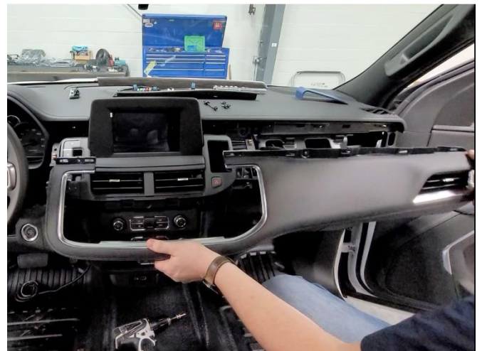
Remove all 7mm head fasteners from top of trim. Remove trim from vehicle.
