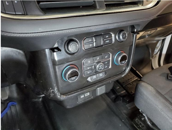
Reattach previously removed dash trim.
