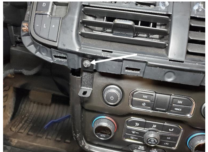
Attach lower dash mounting bracket as shown using previously removed fasteners.
