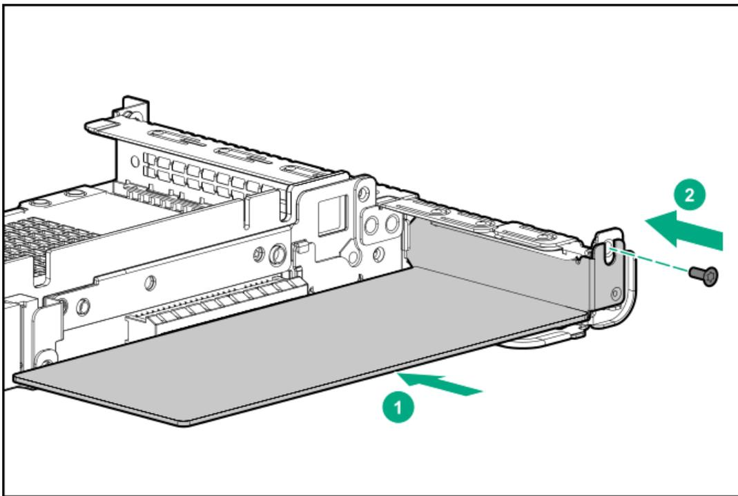
10. Install the primary PCI riser cage.
