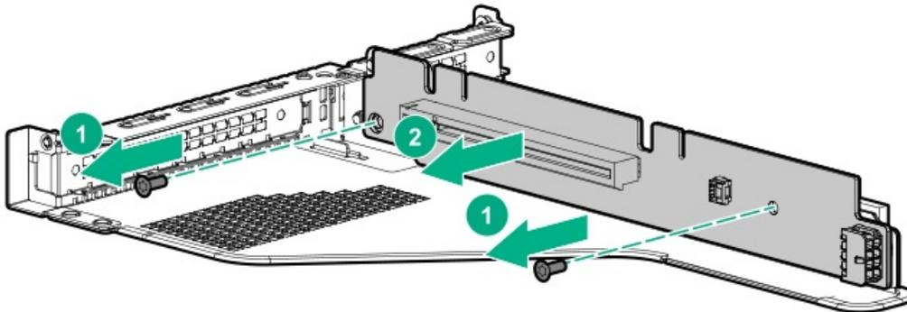
10. Use a T-15 Torx screwdriver to install the riser provided in the kit in the primary PCI riser cage.
