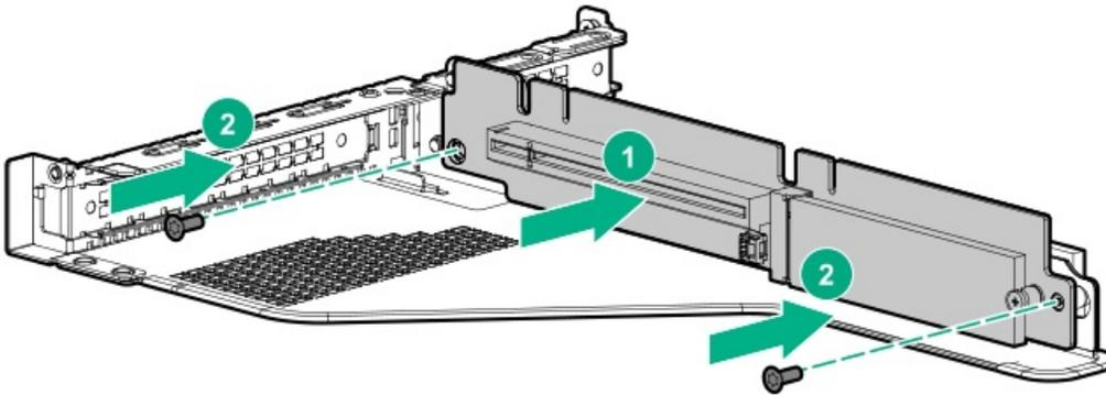
9. Remove the screw securing the standoff on the riser.
