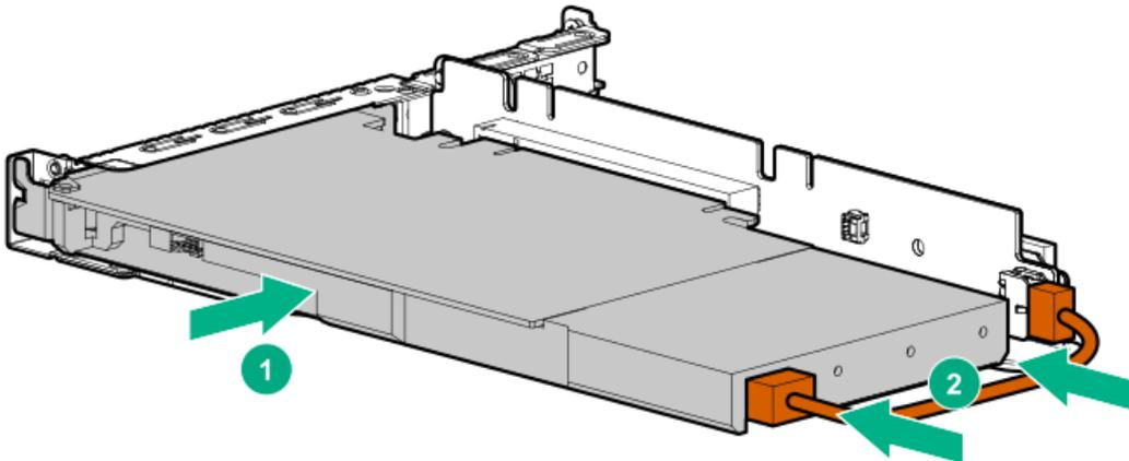
10. If the card requires rear support, install the GPU support bracket.
