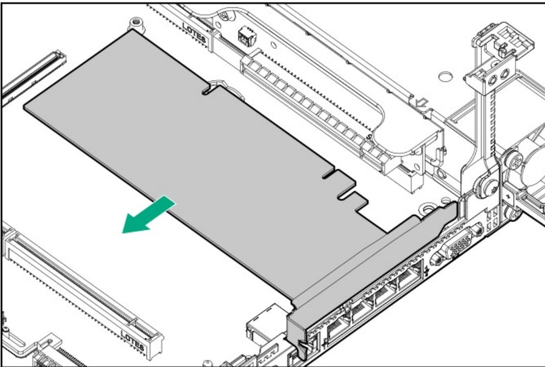
9. Remove the primary PCI riser cage ([Remove the primary PCI riser cage](#)).
