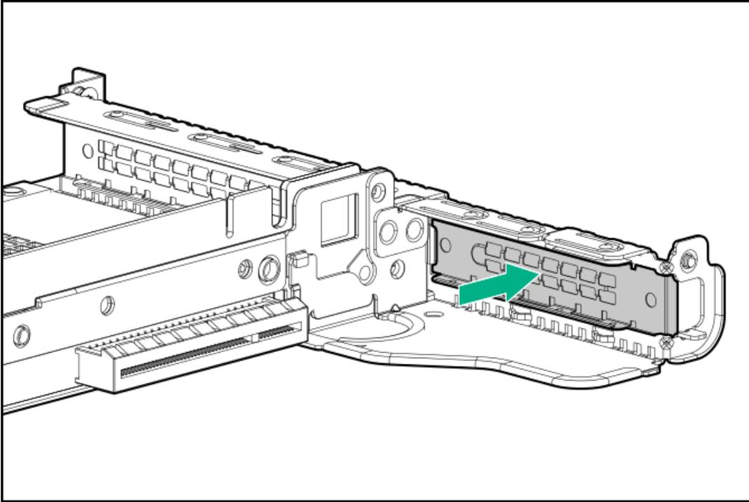
13. Install the DSC-25 card into the PCIe slot.
