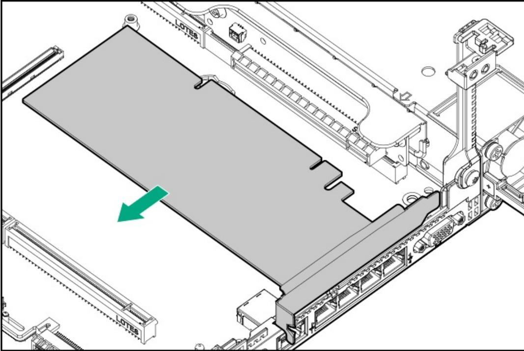
10. Remove the PCI riser cage.
