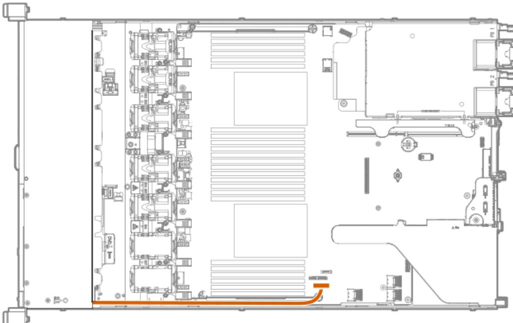
8. Using a Torx T-10 screwdriver, remove the Power/UID/USB assembly.
