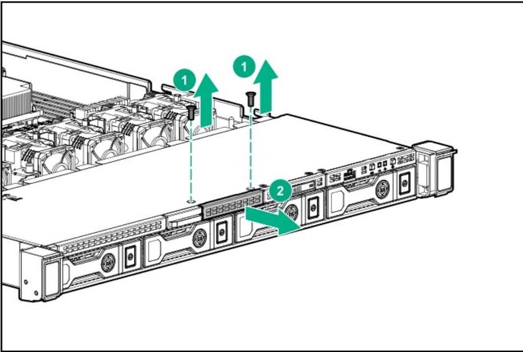
6. Install the 4 LFF display port/USB module.
