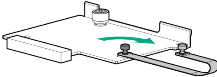
12. Remove the PCIe blank from slot 1 on the primary riser cage.
