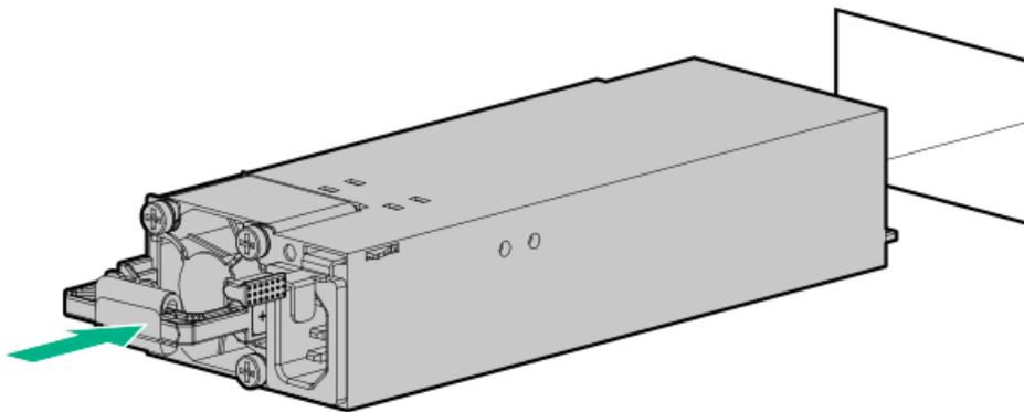
5. Connect the power cord to the power supply.
