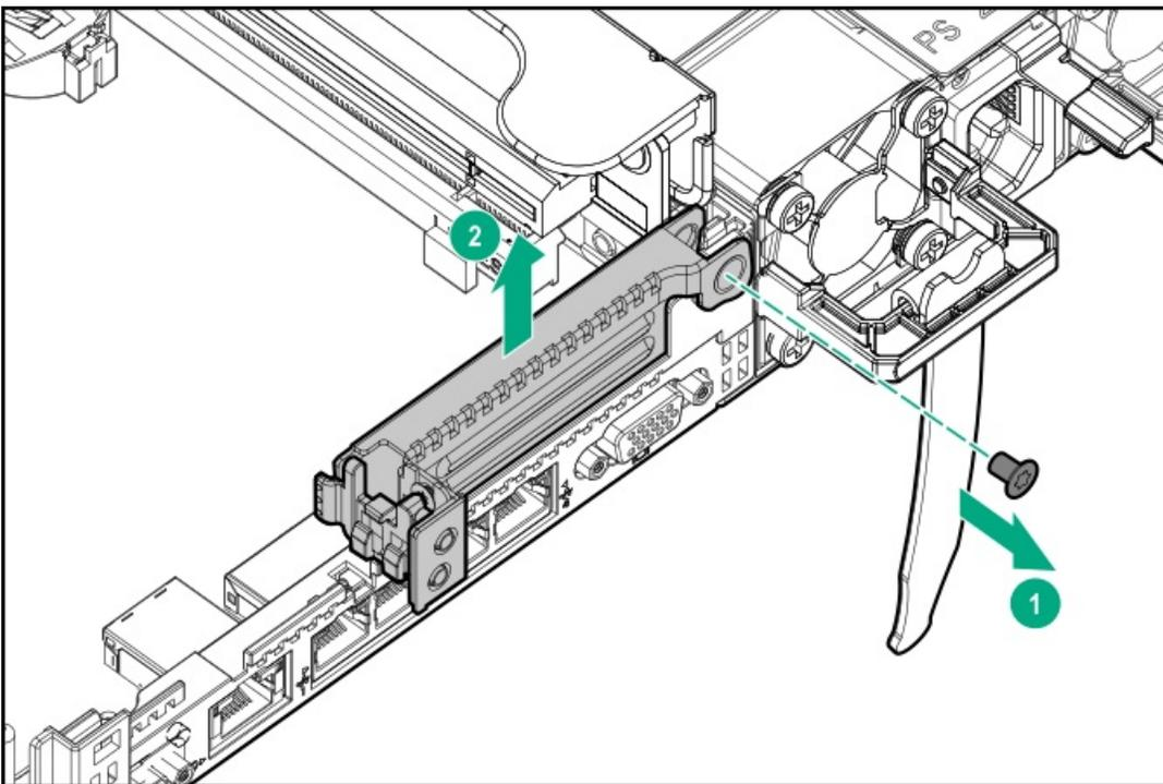
9. Install the full height PCIe x16 riser cage latch.
