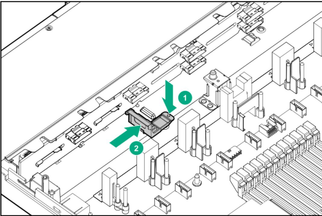
6. Slide the energy pack into the left retainer, and then install the right retainer.
