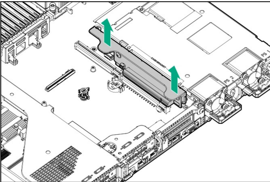
8. Install the secondary full-height PCI riser cage ([Installing a secondary full-height PCI riser cage option](#)).
