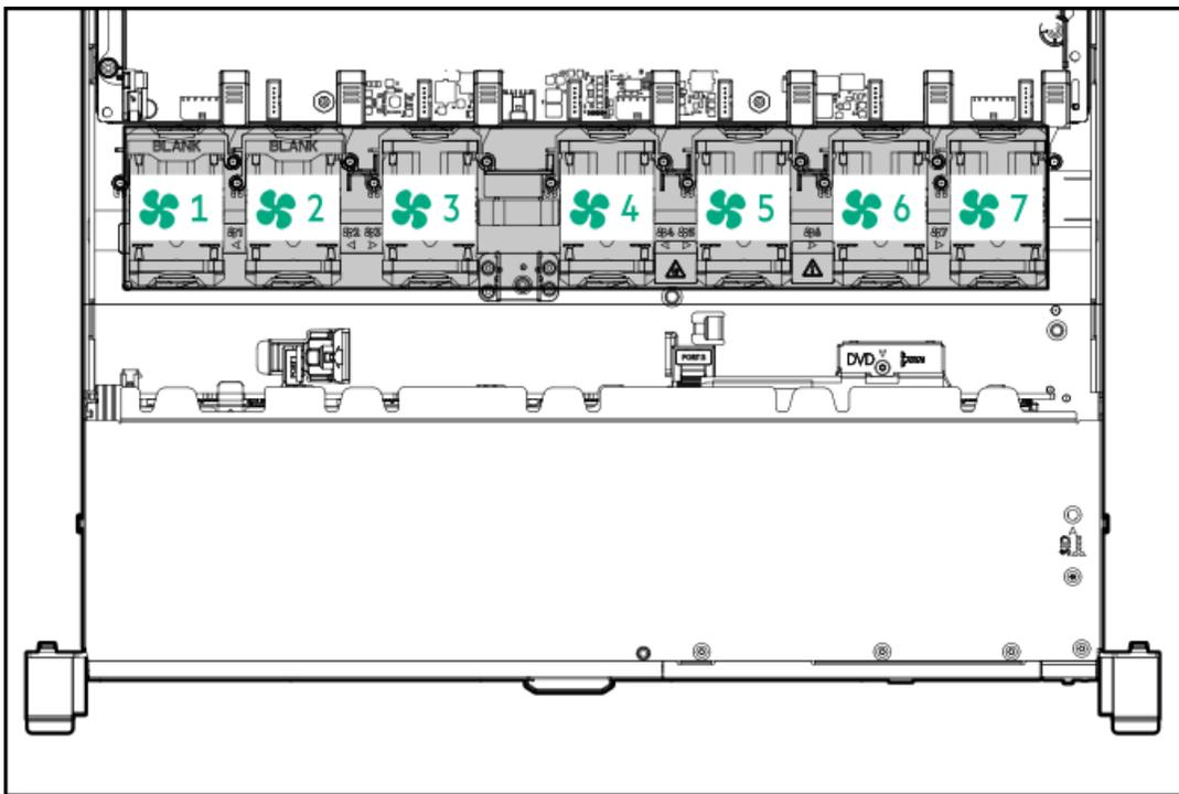
The loss of a single fan rotor (one standard fan) causes loss of redundancy. The loss of two fan rotors (two standard fans or one high performance fan) causes the server to initiate a shutdown.
