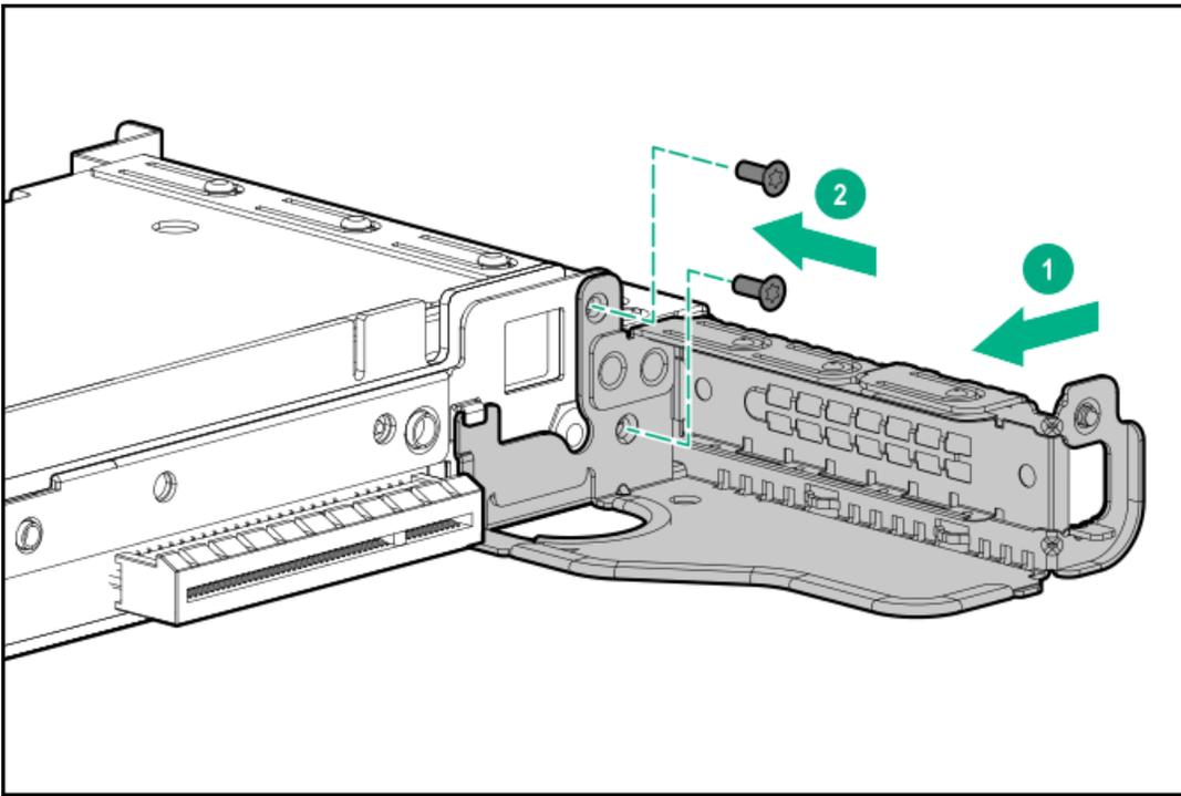
12. If needed, install an expansion board.
