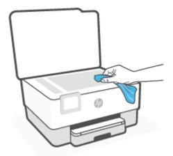
**CAUTION:** Use only glass cleaner to clean the scanner glass. Avoid cleaners that contain abrasives, acetone, benzene, and carbon tetrachloride, all of which can damage the scanner glass. Avoid isopropyl alcohol because it can leave streaks on the scanner glass.
