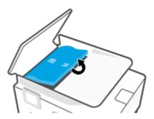
4. Pull any jammed paper out under the rollers.
