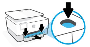
Remove the input tray by pulling it all the way out of the printer.
