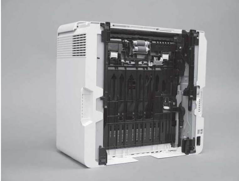
Figure 6-18 Place the printer bottom-side face forward
