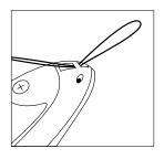
**Step 1:** Pull security cable through the wrist strap eyelet.
