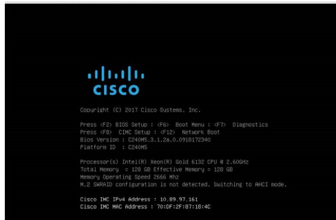
Figure 8: Press F8 at the CIMC Boot Screen
