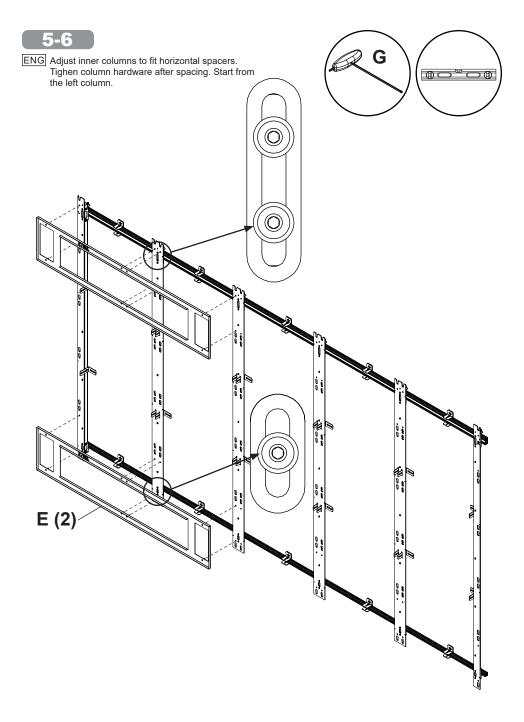
ENG Continue adjusting inner columns to fit horizontal spacers until all are level. Tighen column hardware after spacing
