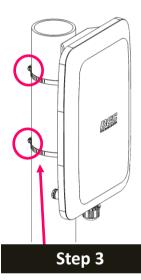
Use a flat-head screwdriver to turn the head of the screw clockwise to tighten the clamps.
