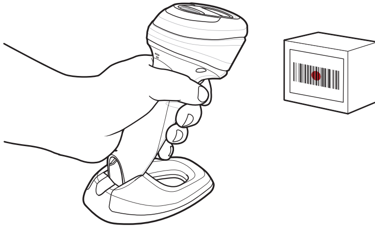
Figure 11 Scanning in Hand-held Mode
