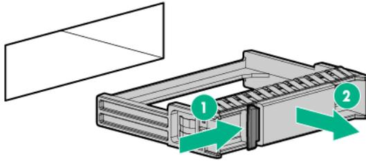
3. Press the Do Not Remove button to open the release handle.
