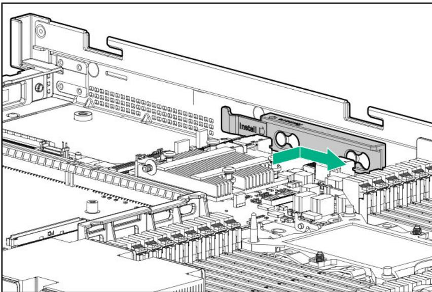
11. Install the riser cage (**Install the primary PCI riser cage**).
