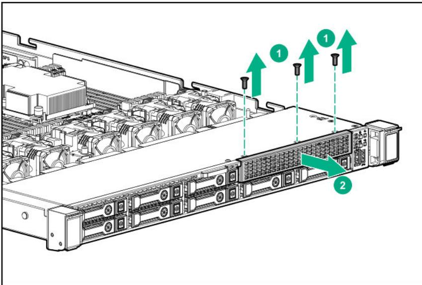
7. Use a T-10 Torx screwdriver to install the 2 SFF NVMe drive cage.
