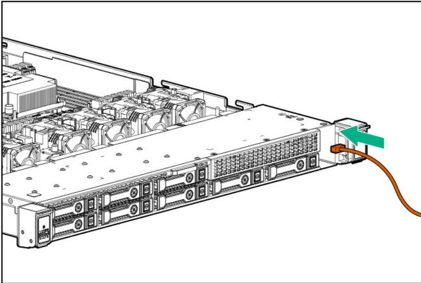
10. Install the SID module into the front panel. Using a T-10 Torx screwdriver, secure the module to the chassis with the screws from the kit.
