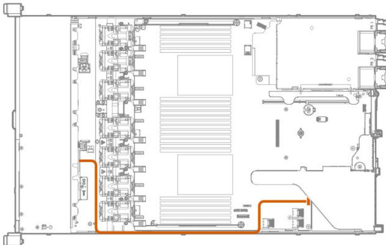
9. If needed, install an optical drive (**Installing an 8 SFF optical drive**).
