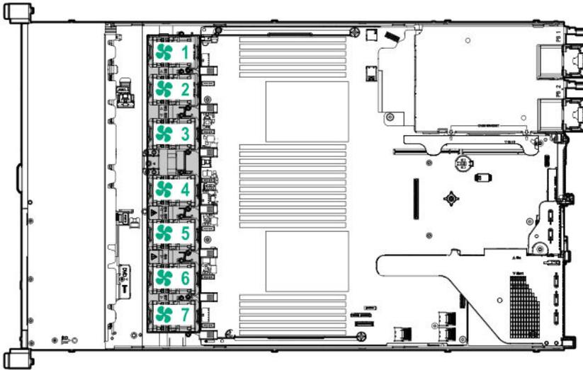
The loss of a single fan rotor (one standard fan) causes loss of redundancy. The loss of two fan rotors (two standard fans or one high-performance fan) causes the server to initiate a shutdown.
