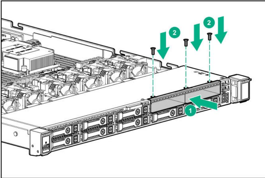
8. Remove the primary PCI riser cage (**Remove the primary PCI riser cage**).
