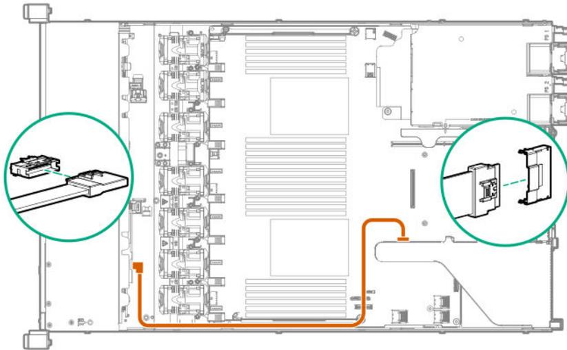
13. Install the primary PCI riser cage.
