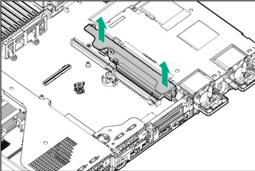
8. Lift and remove the secondary riser cage latch.
