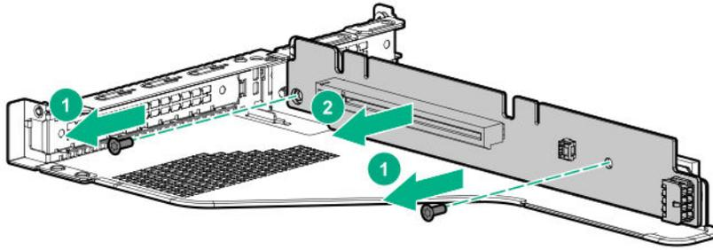
8. If installed, remove the slot 2 bracket from the primary riser cage.
