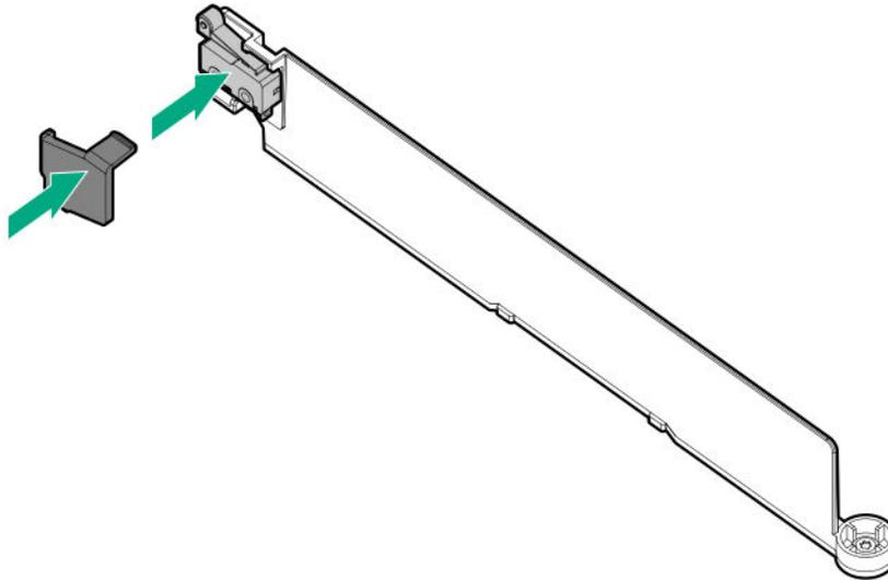
8. Use a T-15 Torx screwdriver to install the DIMM guard, and then connect the cable to the system board.
