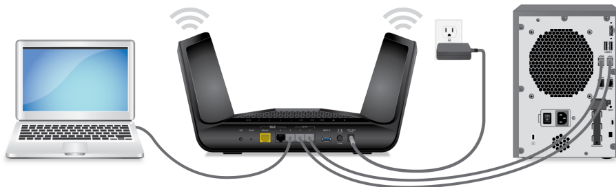
Figure 8. Ethernet port aggregation to a LAN device
