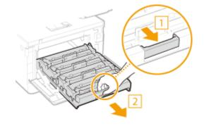
**3** Pull the target toner cartridge straight up and out of the machine.
