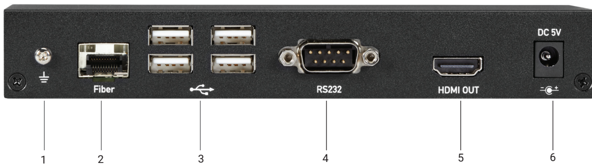
FIGURE 2-10. SINGLE-HEAD FIBER RECEIVER BACK PANEL
