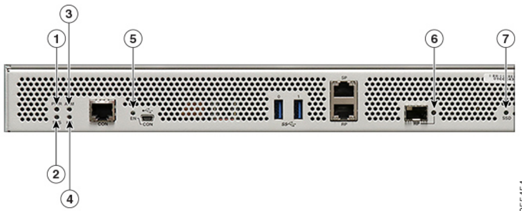
Figure 4: Cisco Catalyst 9800-40 Wireless Controller LEDs
