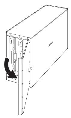
**3** Push the failed drive's cartridge up and remove it from the LinkStation.
