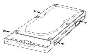
7 Insert the new drive back into the empty slot.
