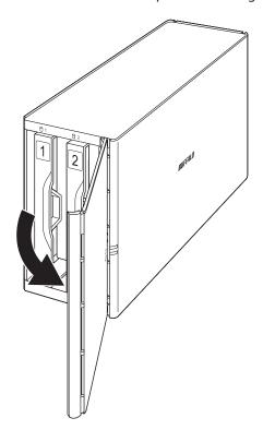
$\boldsymbol{3}$  Push the failed drive's cartridge up and remove it from the LinkStation.
