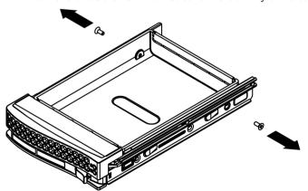
2. Remove the dummy drive from the hard drive carrier and place the hard drive carrier on a flat surface.
