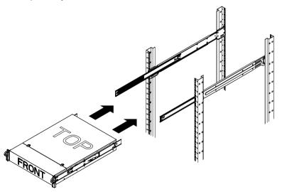
Installing the chassis in a Telco type rack
