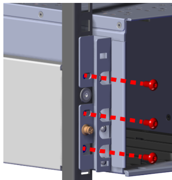
Figure 168: Chassis Screw Removal
