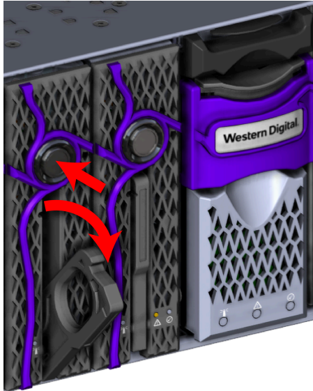
Figure 120: Device Blank Release Operation
