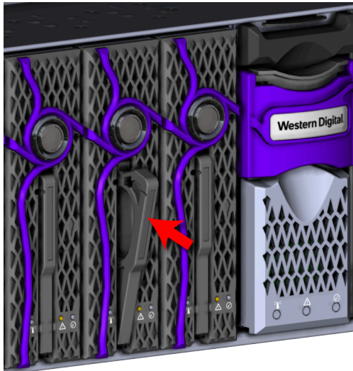
Figure 185: Secure Device Blank
