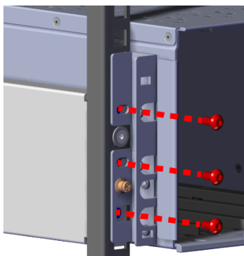
Figure 127: Chassis Screw Removal
