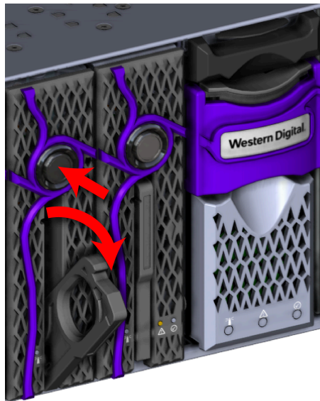
Figure 111: OpenFlex F3100 Release Operation
