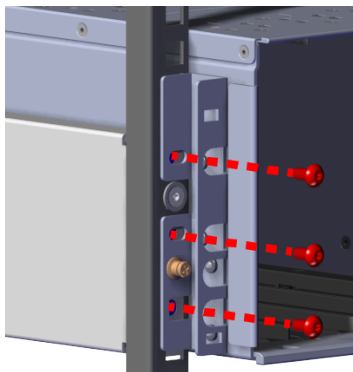
Figure 168: Chassis Screw Removal
