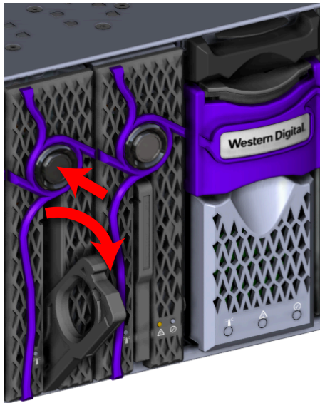
Figure 159: Device Blank Release Operation
