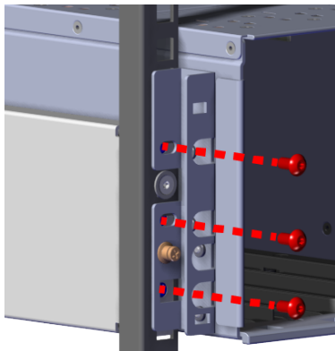
Figure 171: Chassis Screw Installation
