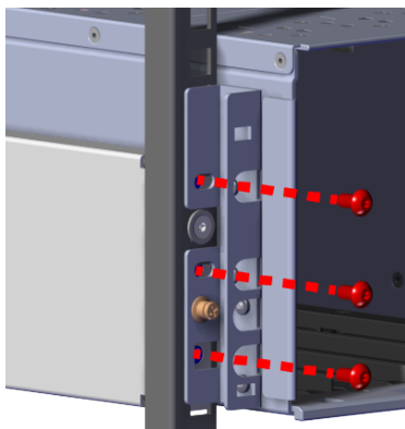
Figure 137: Chassis Screw Installation
