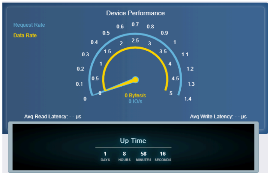
Figure 31: Storage Device Performance Panel
