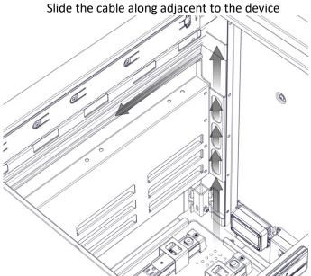
Insert the remaining cables. Evenly space the cables along the rubber grip
