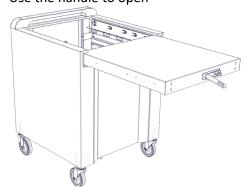
Remove the plastic carry baskets, the mat and the three shelves by lifting on the pull-hole. Lay the shelves on a scratch-proof surface
