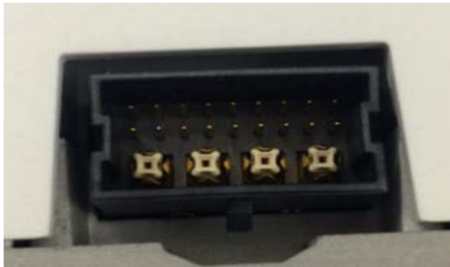
Figure 11 Smart Antenna Connector C9120AXE and C9120AXP Models
