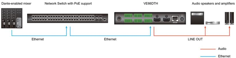
**Note:** Via the VE66DTH, audio speakers and amplifiers that do not support Dante™ networked audio interface can be integrated into a Dante™ networking system.
