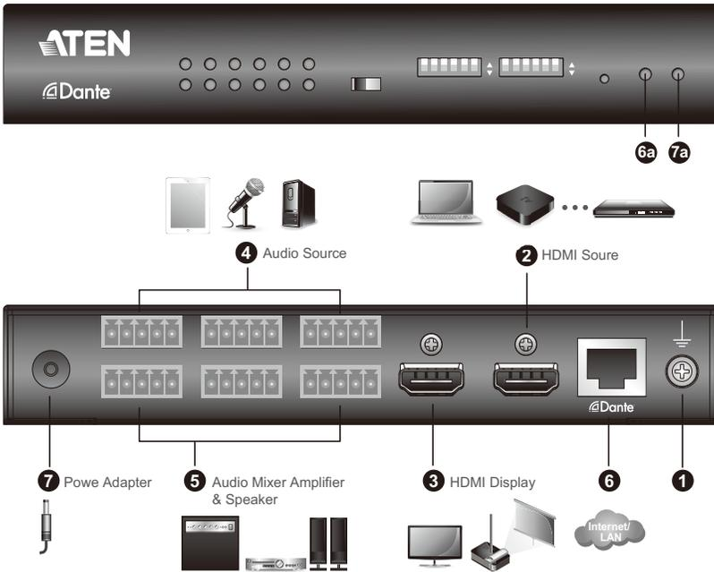
1. Ground the VE66DTH by connecting one end of a grounding wire to the ground terminal and the other end to a suitable grounded object.
