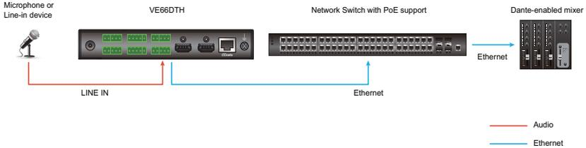
**Note:** The VE66DTH is used to integrate up to 6 analog LINE signals into a Dante™ networking system.
