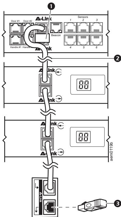
1. Connect sensors and sensor pods to the in and out ports as shown.
