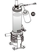
Place your PSU outside of the case and attach it to the pumps 4pin molex connector, turn on the power of PSU and make the rest of the system fills up.
