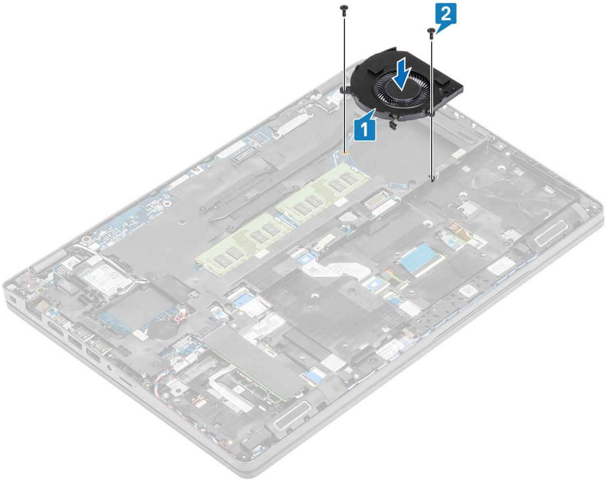
3. Connect the system fan cable to the connector on the system board.
