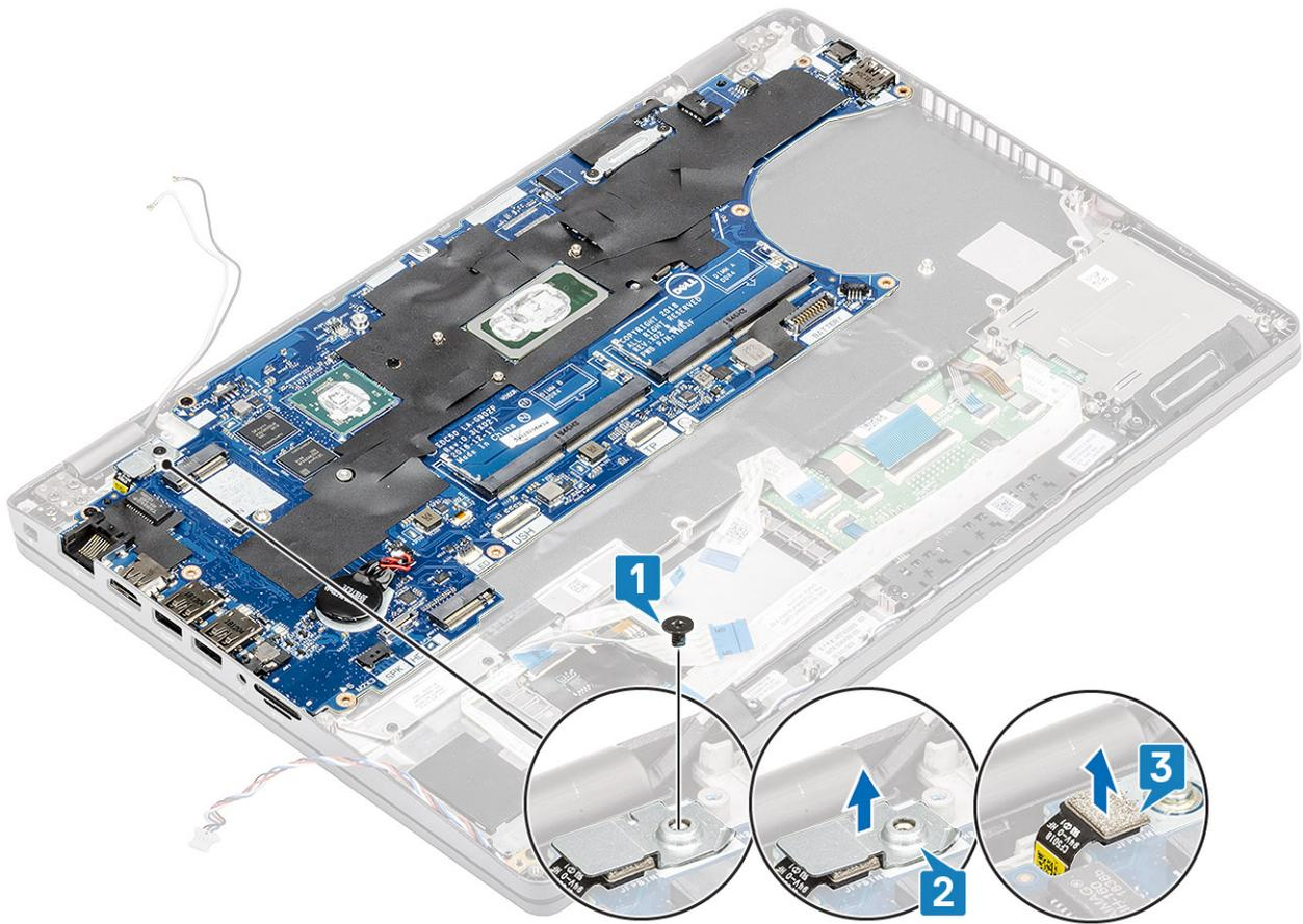
5. Remove the five (M2x3) screws that secure the system board to the computer [1].
