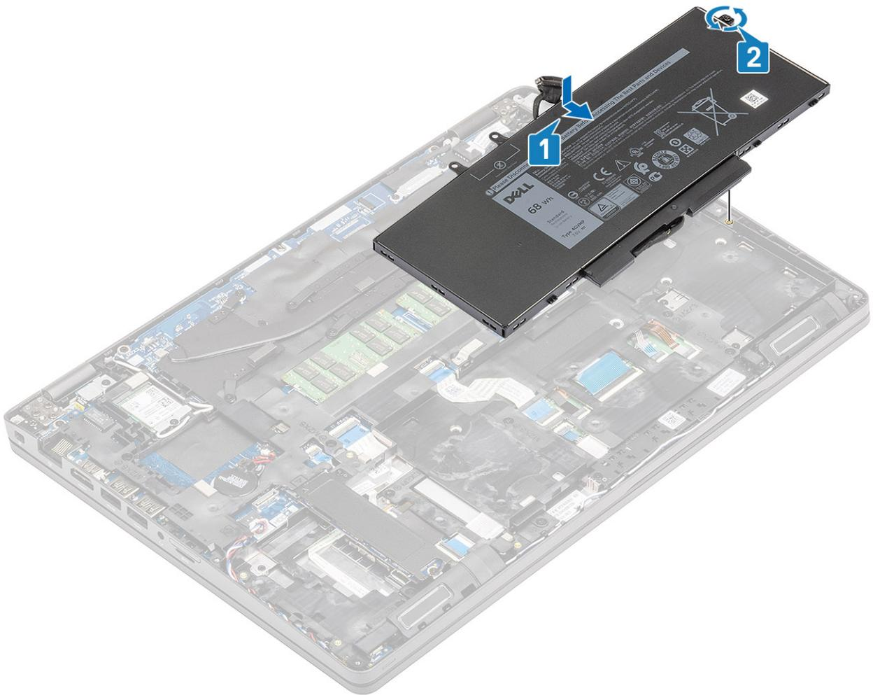
2. Reconnect the battery cable to the connector on the system board.
