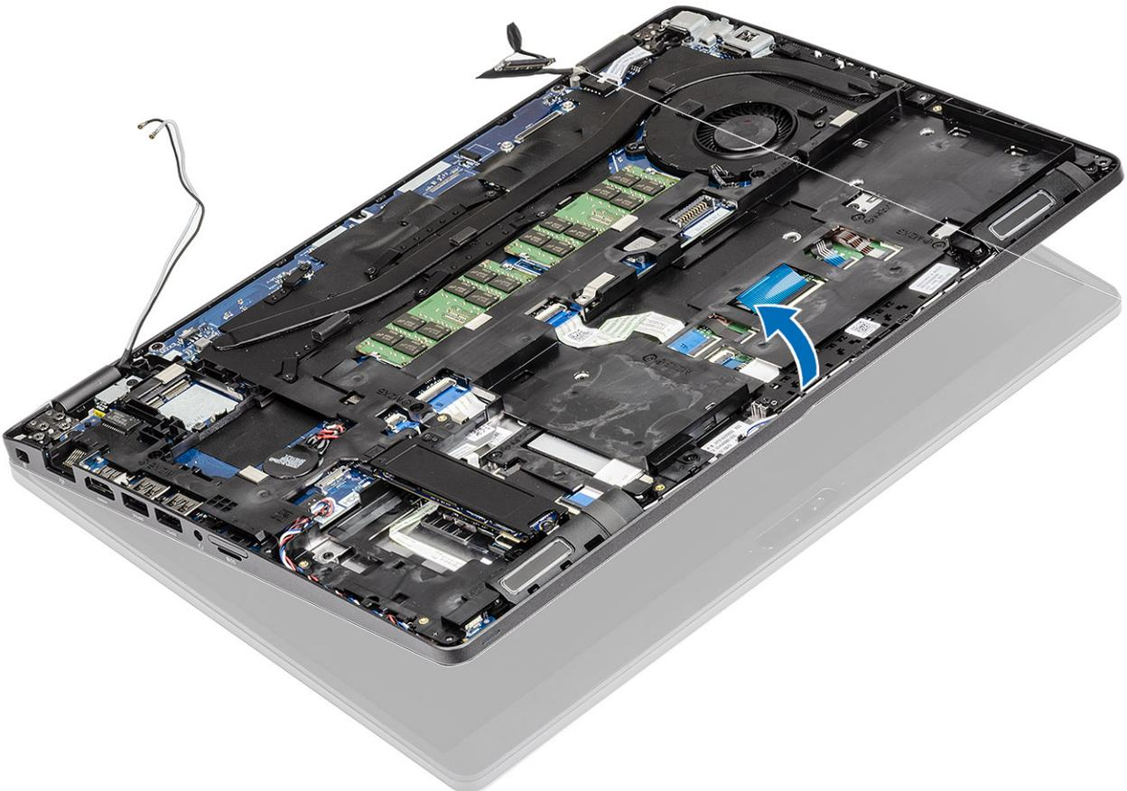
4. Remove the six (M2.5x5.0) display hinge bracket screws that secure the display assembly to the system [1].
