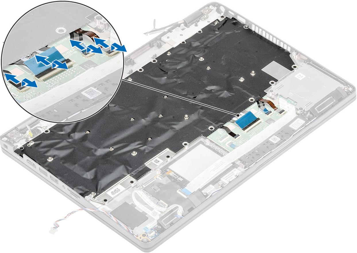
2. Remove the nineteen (M2x2) screws that secure the keyboard [1].
