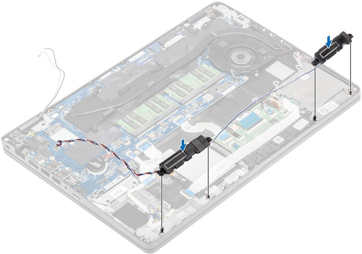
2. Re-route the speaker cables through the routing clips on the computer chassis
