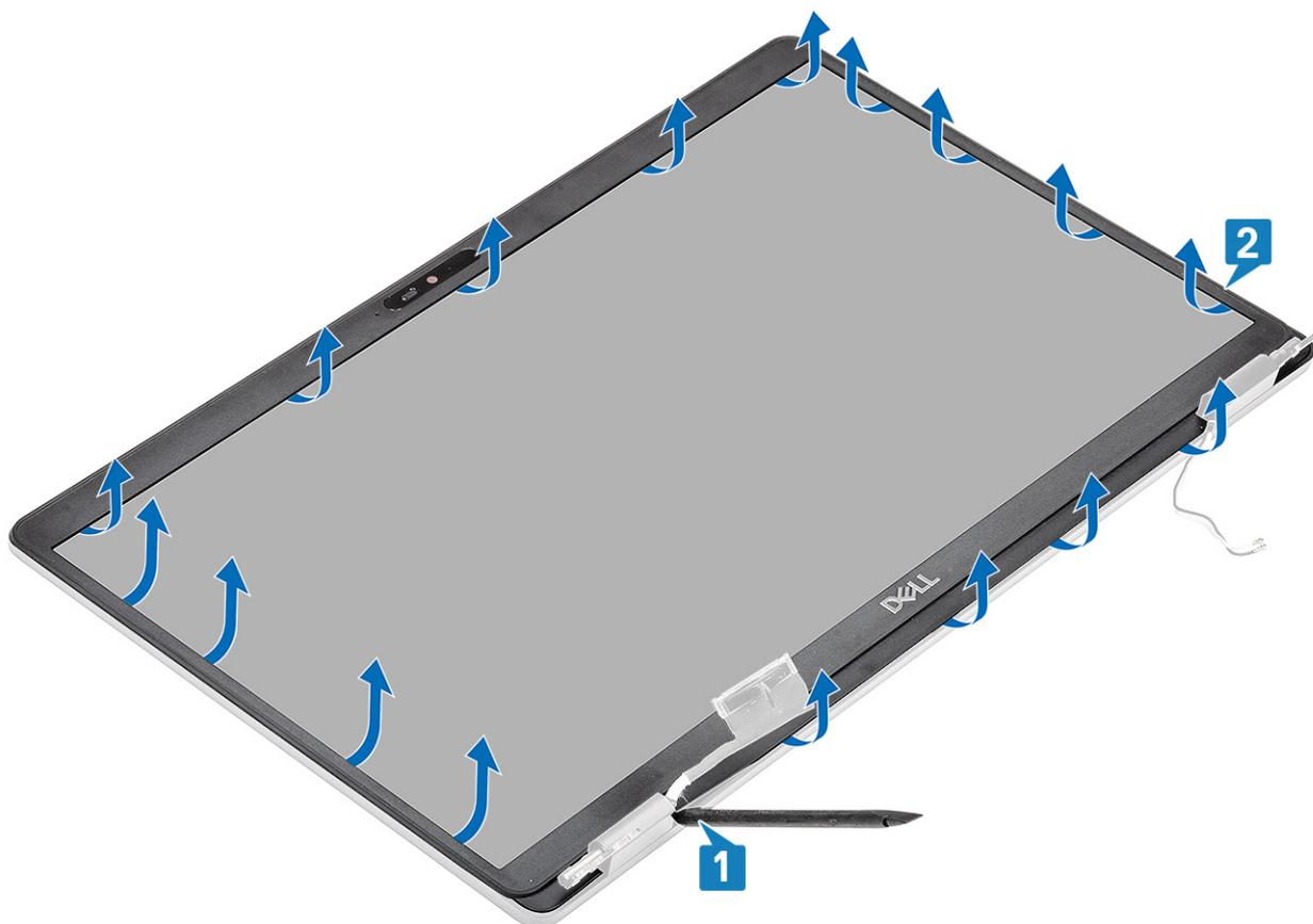
3. Lift the display bezel from the display assembly.
