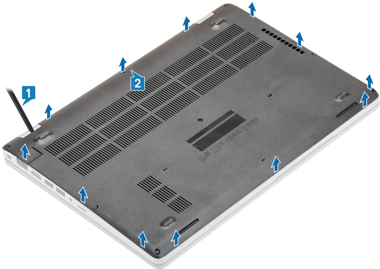
**NOTE:** While removing the base cover, on-site technicians must take care to remove the base cover carefully. There are prying recess points next to the left and right hinges which ease the disassembly procedure. With the help of a plastic scribe, pry open from the top left side of the base cover, continue working your way around the left and right side of the base cover, then remove the base cover from the system.
