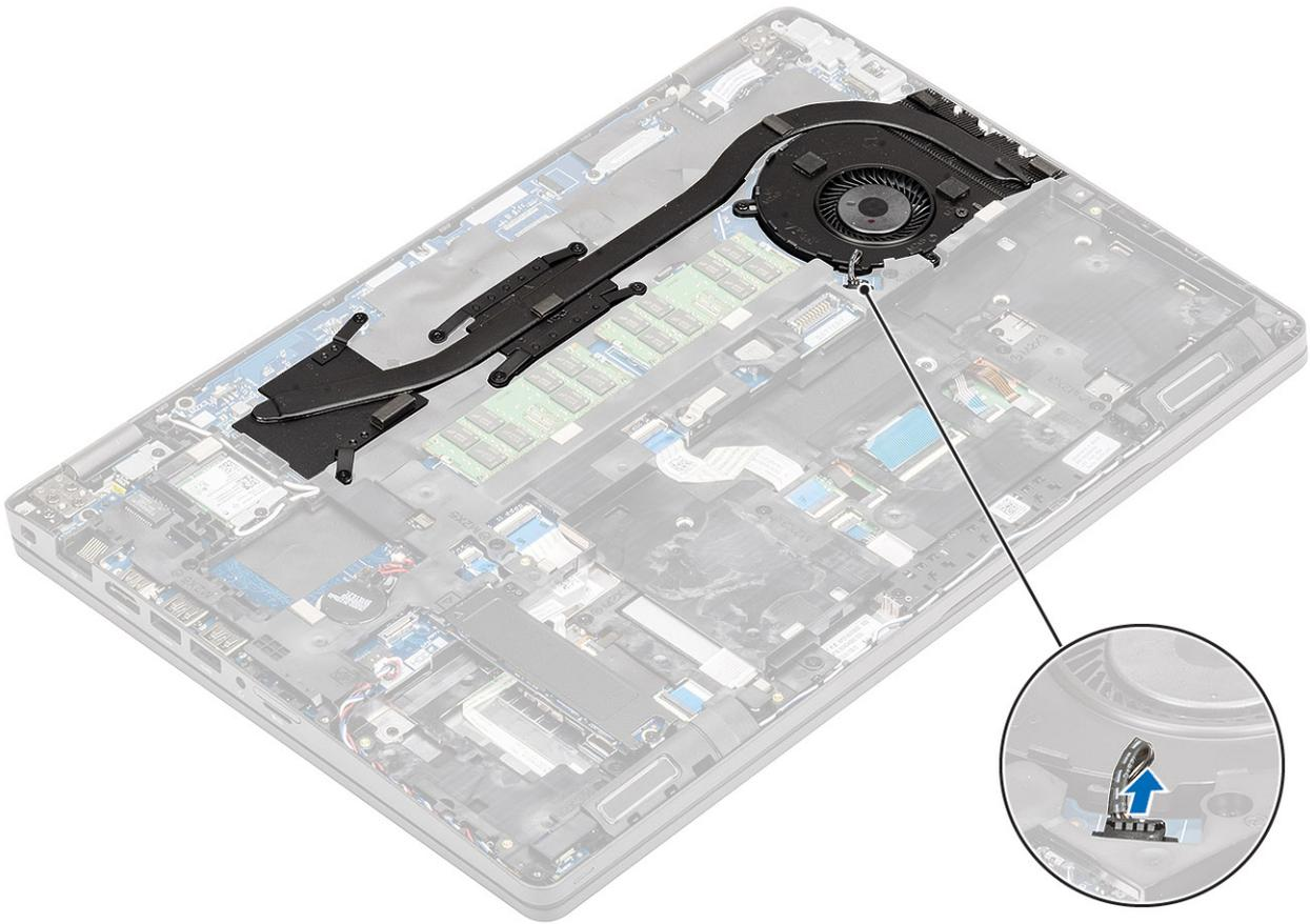
2. Remove the seven (M2x3) screws and the two (M2x5) screws as per the numerical callout on the Heatsink [1].
