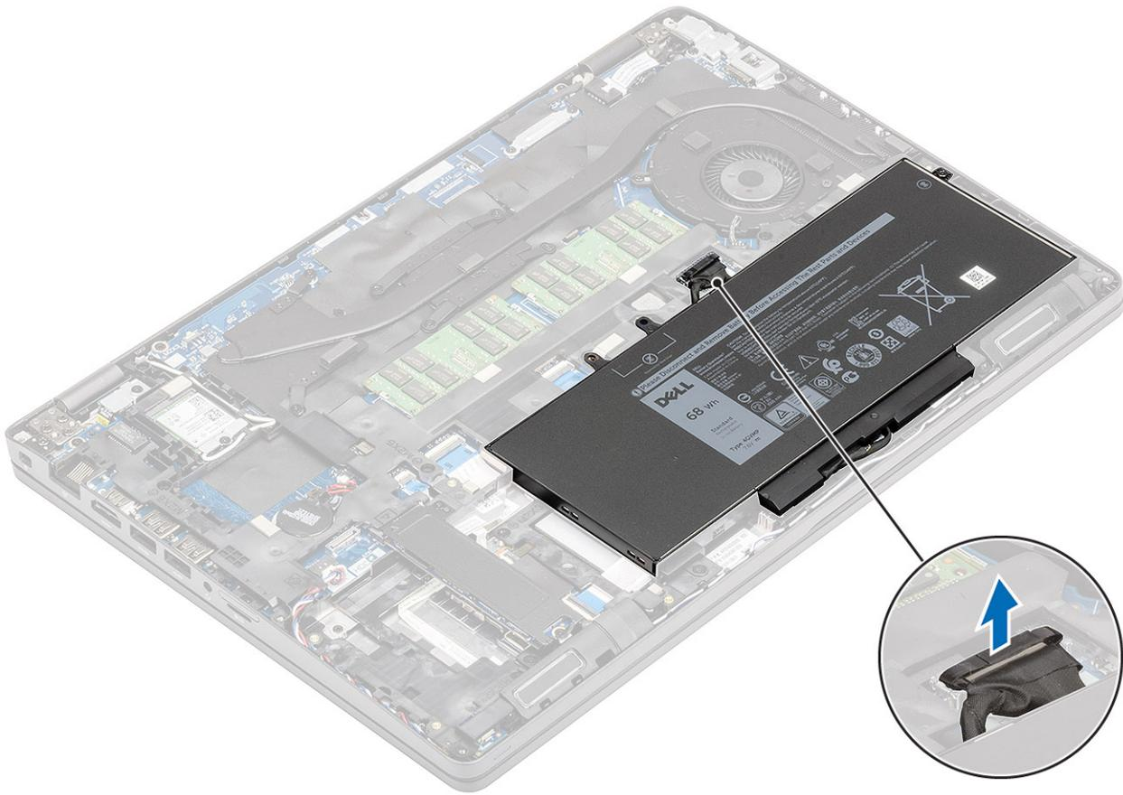
2. Remove the one (M2.0x4.0) screw that secures the battery to the palmrest [1].
