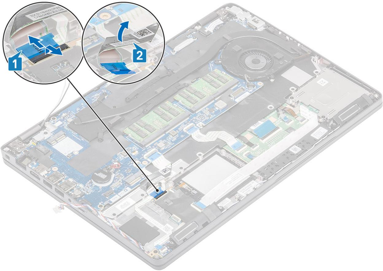
2. Unlock and disconnect the LED board cable from the system board [1].
