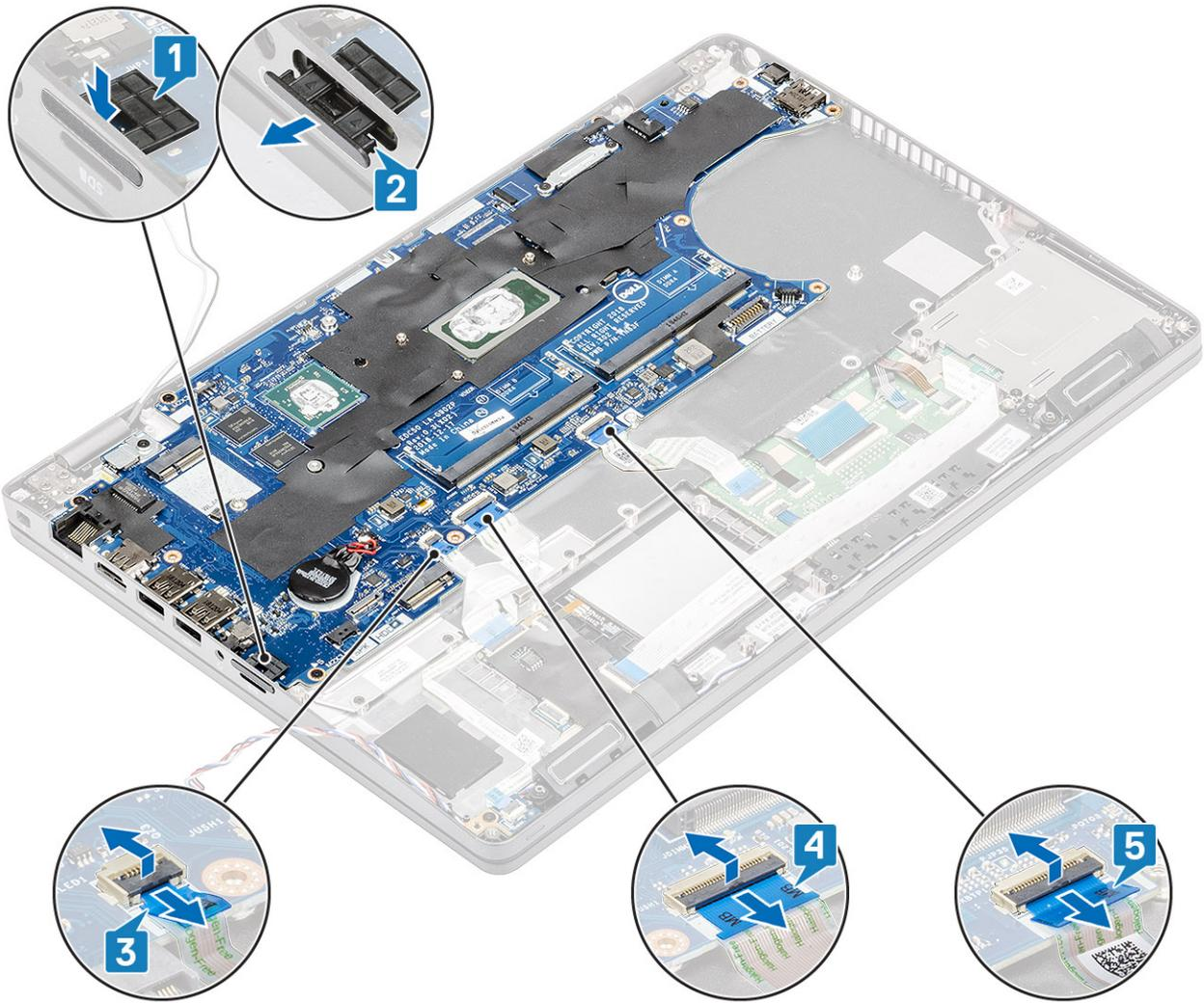
3. Remove the single screw securing the metal bracket to the computer [1] and lift it away from the computer [2].
