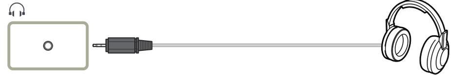
— The headphones or earphones jack supports only the 3 conductor tip-ring-sleeve (TRS) type.
