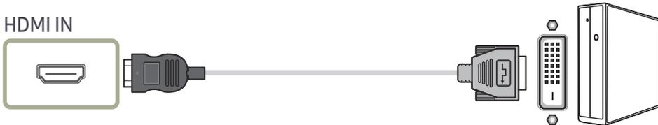
— The audio function is not supported if the source device is connected using the HDMI-DVI cable.
