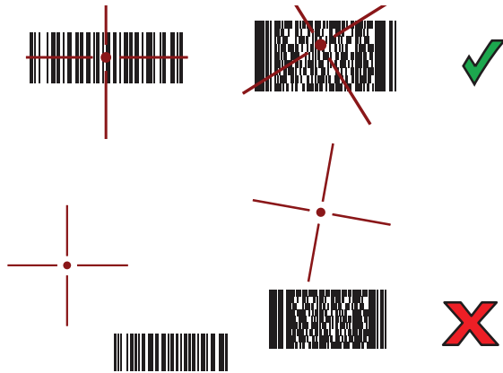
Figure 29 RS5100 Pick List Mode with Multiple Barcodes in Aiming Pattern
