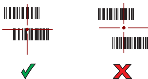
Figure 31 RS6000 Pick List Mode with Multiple Barcodes in Aiming Pattern
