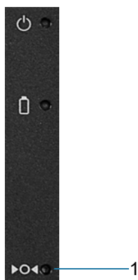
Figure 38 Reset Switch on Front of Tablet
