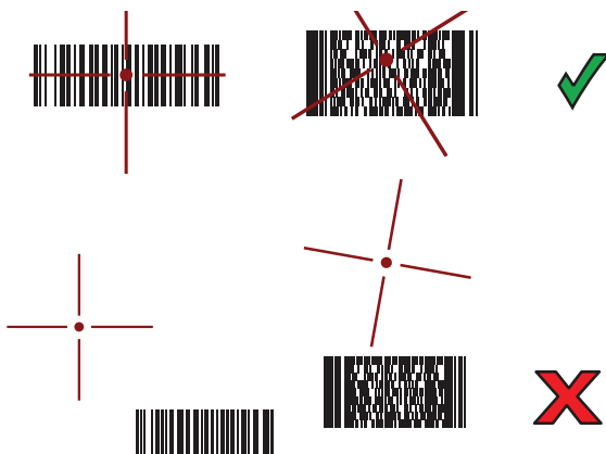
Figure 26 RS507/RS507X Aiming Pattern
