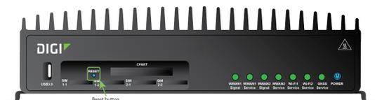
2. Press and hold the **RESET** button perform a device reset. The **RESET** button has two modes:
