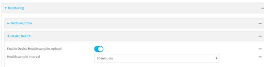
Device health data upload is enabled by default. To disable, click to toggle off **Enable Device Health samples upload**.
