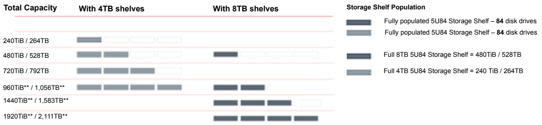
Figure 2-2 Available Flex 5340 Appliance 5U84 Storage Shelf configurations
