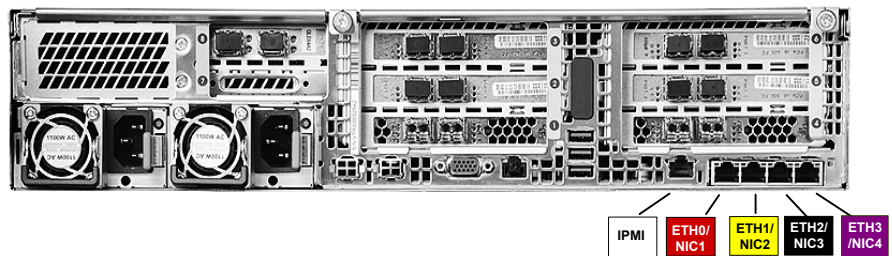
Figure 1-8 5340 Appliance rear port color codes
