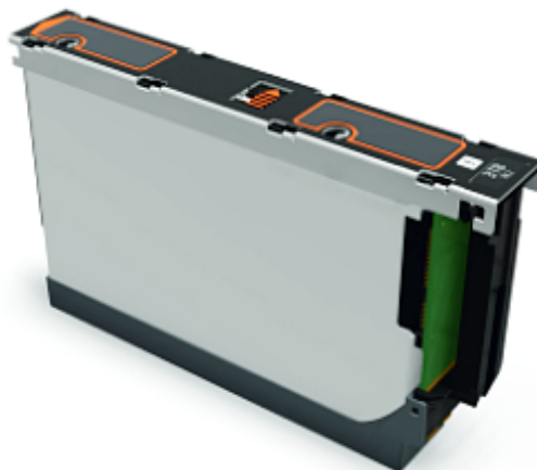
Figure 2-4 Disk Drive In Carrier (DDIC) module
