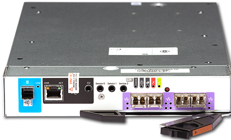
Figure 2-16 Veritas 5U84 Primary Storage Shelf Fibre Channel RAID controller
