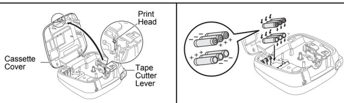
With the LCD facing down, open the Cassette Cover by pressing the grooved tab and pushing in the direction of the arrow, as illustrated.
